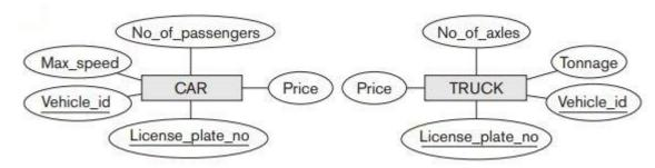
Generalize CAR and TRUCK into the superclass VEHICLE
