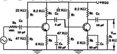
$\beta_1=100$  ,  $\beta_2=150$  ,  $r_{\pi 1}=r_{\pi 2}=1.3~\text{K}\Omega$  ,  $g_{m1}=g_{m2}=50\text{mA/V}$
