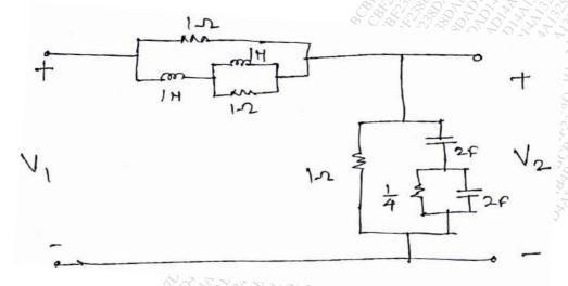
Q.3 (A) In the network of figure, find the voltage  $V_2$  which results in zero current through  $4\Omega$  [10M]
