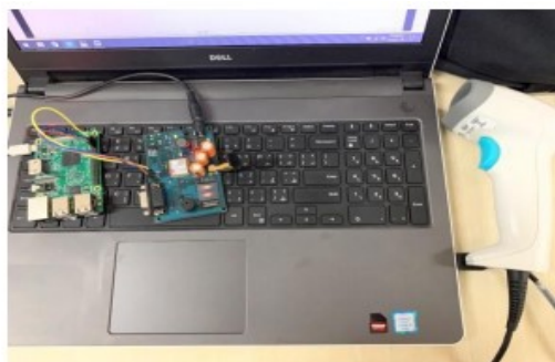
Fig. 6 Raspberry Pi 3, GSM Module and QR code scanner
